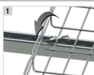
Hook one side of the FS41 into channel support.
