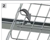
Depress FS41 and hook other side into channel support.
