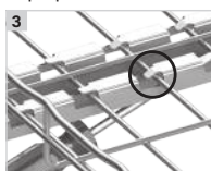
From the underside, depress several tabs using a screwdriver or pliers to secure tray
