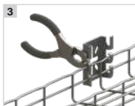
Depress all tabs using a screwdriver or pliers to secure tray
