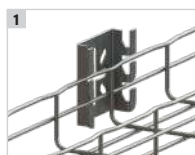
Attach mount to wall
