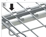
Insert tray into slots
