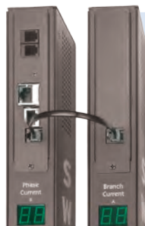
Rear View: network, serial, linking and temperature/humidity inputs
